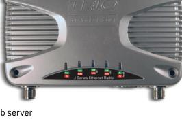
(DHCP, HDP, TCP, MODBUS, DNP3), Auto or Manual DHCP configuration, and dual industry-standard TNC antenna connectors.
