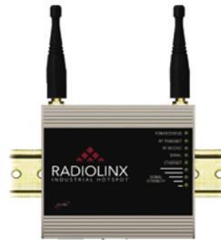
signal strength and much more. Because the radios are based on 802-11.b with TKIP encryption, they offer a secure method of connecting our laptops to our network from the field. The two antennas on each radio provide antenna diversity to help reduce the effects of spurious, reflected signals.
